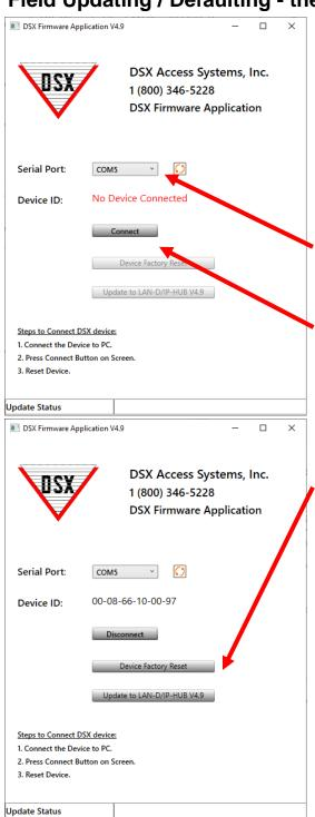
Use the following steps to Flash update or to reset the LAN-D and IP-HUB. Connect the module to 5 or 12VDC. Using a DSX-USB module, connect the RS-485 port of the DSX-USB Module to the RS-485 port of the LAN-D or IP-HUB. Be sure and cross the transmit and receive terminals. TX+ to RX+ and TX- to RX-.
