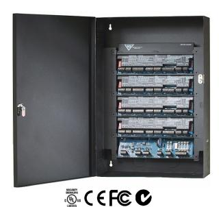
Each DSX-1048PKG includes a DSX-1040E Enclosure, a DSX-1040CDM Communications Distribution Module and 4 DSX-1042 Intelligent Controllers. Each DSX-1048 provides 8 Reader Ports, 32 Inputs and 16 Outputs. Each DSX-1042 has a 12V fused power Output for its Card Readers and Keypads. The DSX-1042 contains an RDC186 Processor, 512K of RAM, 512K of Flash ROM and a Real Time Clock. Removable terminal blocks allow all Door and field wiring connections to be made easily.
