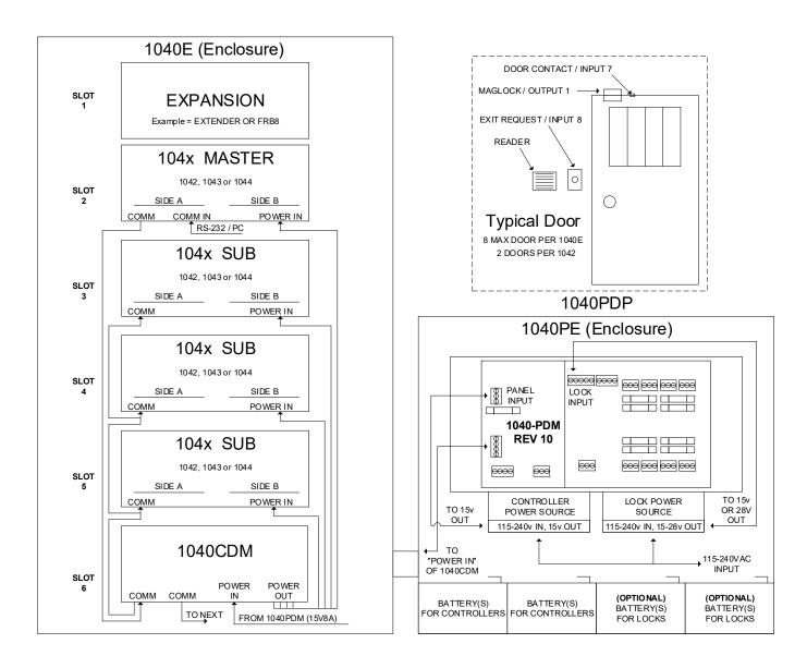
The DSX-1048PKG includes a DSX-1040E Enclosure, a DSX-1040CDM Communication Distribution Module and 4 DSX-1042 Intelligent Controllers. This provides 8 Reader Ports, 32 Inputs and 16 Outputs. The DSX-1048PKG comes complete with 32 - 1K ohm EOL Resistors, Lock & Key, Wire Ties, Tamper Switch, an External Power Indicator and a DSX-1040PDP Power Distribution Panel.
